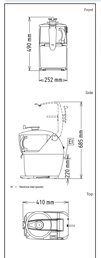
Electric Supply voltage: 200-240 V/1N ph/50/60 Hz Electrical power, max: 1.3 kW **Total Watts:** 1.3 kW Capacity: Performance (up to): 550 kg/hour 5.5 litres Capacity: **Key Information:** External dimensions, Width: 252 mm 485 mm
